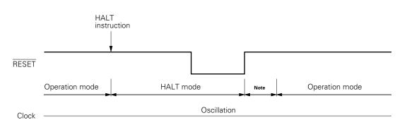
When the RESET signal is applied to release the HALT mode, the RESET input makes a transition from low to high, then an operation mode is entered.
