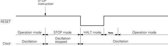
As soon as the RESET input makes a transition from high to low in the STOP mode, the system clock starts generating clock pulses.
