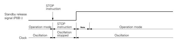
**Note** The HALT mode remains effective in this period, waiting for the generation of clock pulses to settle. An operation starts after eight clock pulses on the XIN pin are counted.
